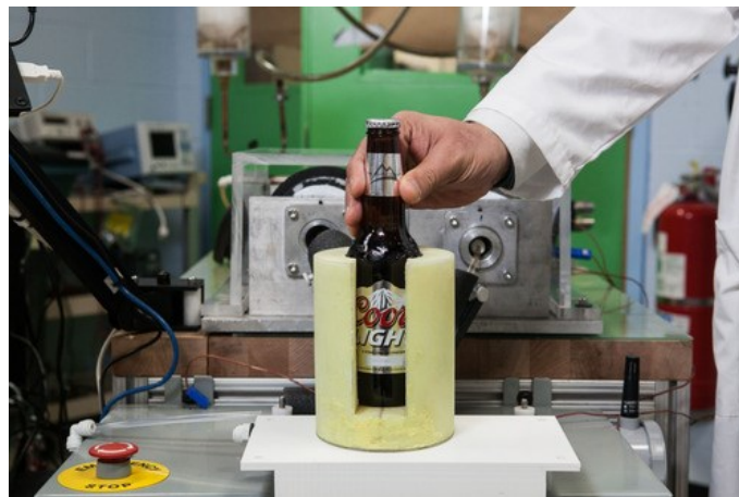
Fig. 1.29. Prototype of the magnetocaloric refrigeration system based on the Ni-Mn-Ga alloy developed by General Electric and Oak Ridge National Laboratory (derived from [495]).
