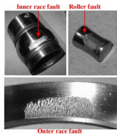
FIGURE 3.5: Different faults of rolling element bearings [114].
