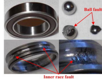
FIGURE 3.2: Different faults of rolling element bearings [97].
