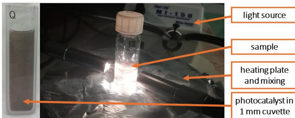
Figure 60. AuPdNRs-CNFs photocatalyst in a 1 mm cuvette and representative photograph of the photocatalytic setup.
