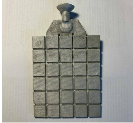
Fig. 7.1 Exemplary plate casting for testing casting parameters; a plate consists of small cubes
