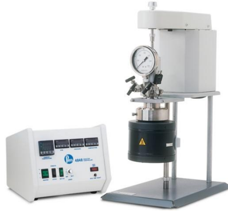
Fig. 11. Image of utilized Parr reactor for the hydrothermal functionalization of CNF [185].
