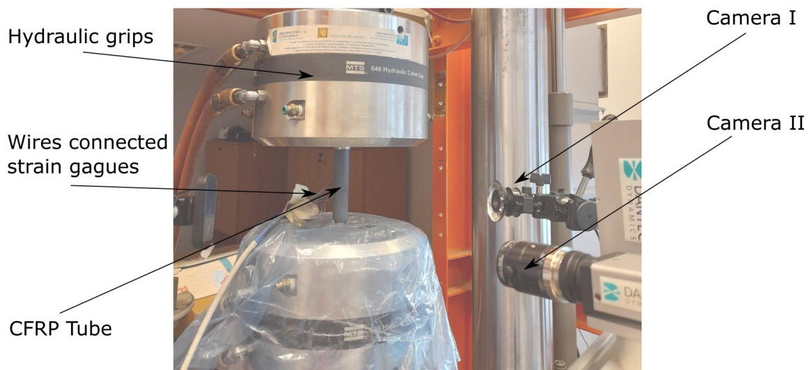
Fig. 19. Experimental setup used in the presented research equipped with a camera I used for sample monitoring, camera II as part of the DIC system used, and strain gauges. Graphic by the author, first published in [11] under https://creativecommons.org/licenses/by/4.0/
