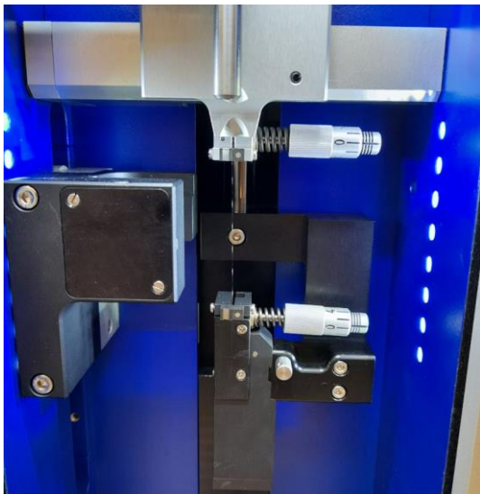
Fig. 13. a) Experimental TexTechno setup for testing single fiber; b) single carbon fiber during the test; c) obtained results from the test as a function of force vs. elongation
