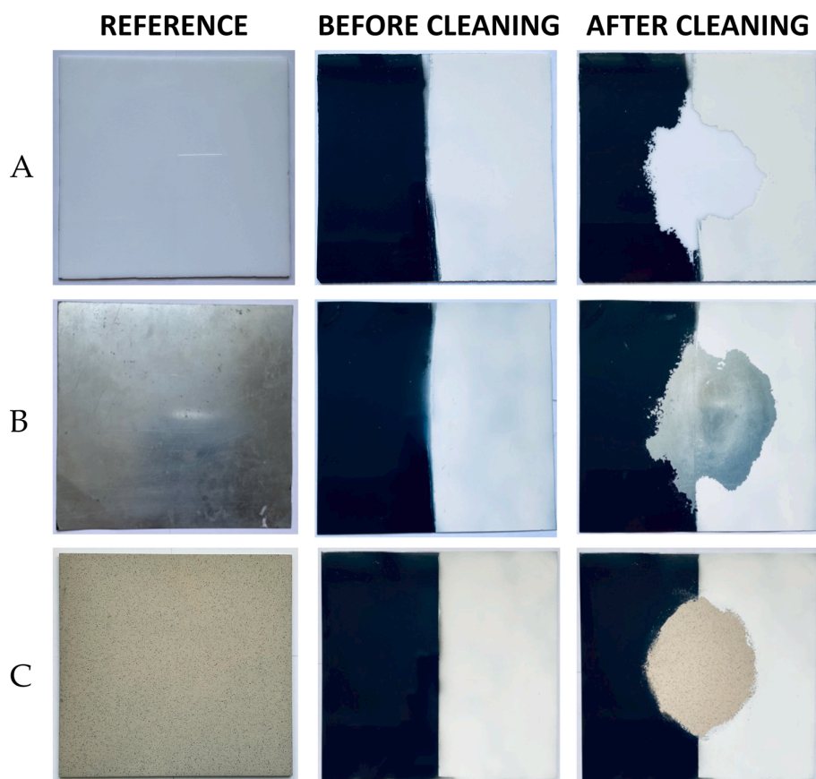
Fig. 7. Exemplary samples of surfaces sensitive to mechanical cleaning as evaluated by in situ detergent tests: (A) acrylic glass, (B) steel, and (C) ceramic tile.
