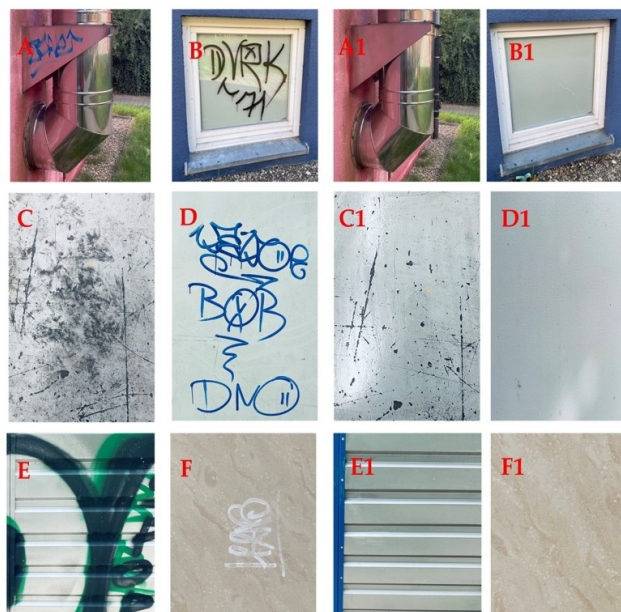
Figure 6. Different surfaces were cleaned with green nanostructured fluid no. 1 in the city of Wrocław: (A) stainless steel; (B) window glass; (C) concrete floor; (D) concrete floor with protective coating; (E) aluminum facade; (F) ceramic tiles.
