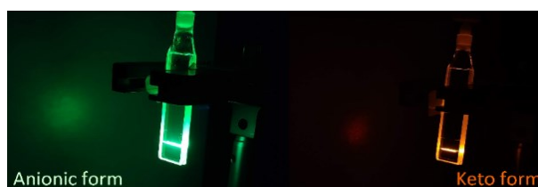
Figure 6.2.10. Stimulated emission spectra of anionic and keto forms in 1.5 mM HBT-CF3-4,6-TMS /toluene solutions, along with photographs taken during experiment.
