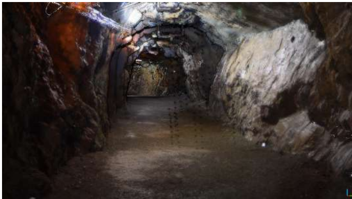
FIGURE 2.5. TLS point cloud of an underground tunnel textured with an DSLR image (Trybała, 2021)
