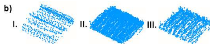
Figure 21. Point cloud resolution comparison for object (b)—isometric views.
