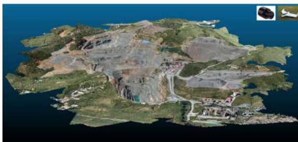
FIGURE 2.1. Perspective view of a photogrammetric 3D reconstruction of an open pit mine (Chen et al., 2015)
