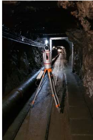
Figure 2. Reference measurements with a Riegl Vz-400i
