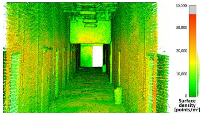
Figure 10. Point cloud density—rotating lidar.
