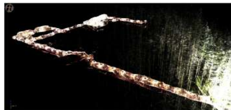
Figure 3: Registered reference point cloud of the entire underground complex.
