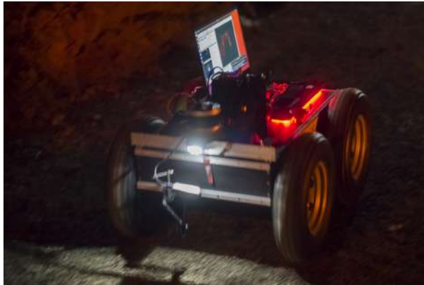
Figure 3. Mobile robot equipped with a Velodyne VLP-16 and a laptop for data collection
