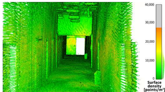
Figure 11. Point cloud density—tilting lidar.
