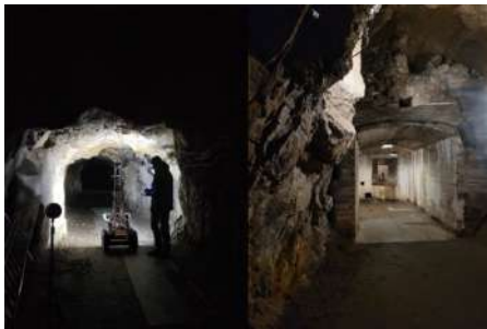
Fig. 18 Challenges for SLAM in the underground environment: uneven illumination, lack of visual features (left); changing types of geometry: passage from an unstructured tunnel to a concrete corridor (right)
