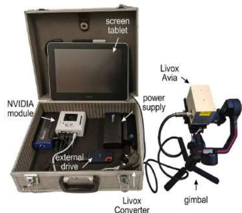
Figure 2. Assembled PoLiMap and its equipment.
