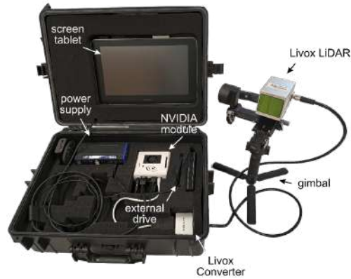
FIGURE 3.9. The proposed mobile mapping system PoLiMap (Trybała et al., 2023b)
