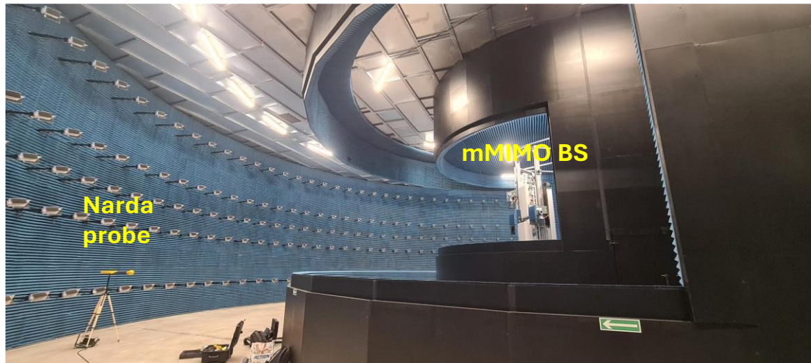
Figure 7-1 OTA chamber with mMIMO BS and EMF meter (Nokia Solution and Networks Laboratory in Wroclaw).
