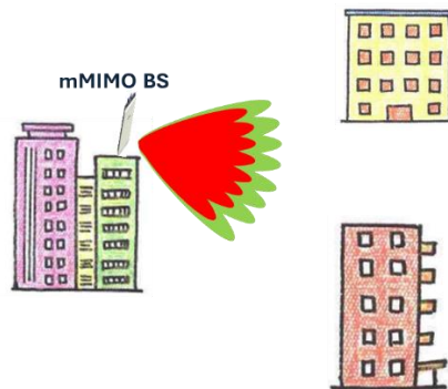
Figure 8-1 Illustration of EIRP control without segments (green – EIRP control disables, red – EIRP control enabled).
