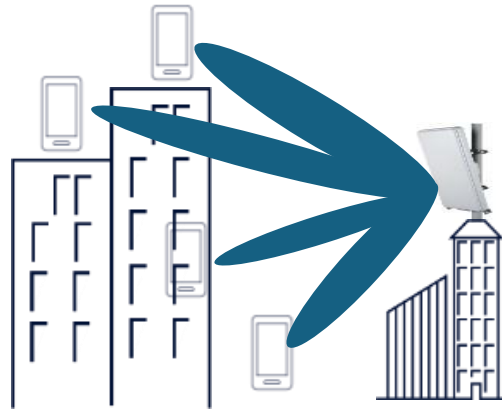
Figure 1-3 Illustration of massive MIMO principles: spatial (angular) separation of four UEs to provide multiplexing gain on orthogonal beams.
