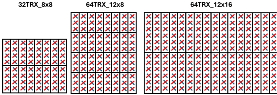
Figure 3-5 Antenna Array configurations used in simulations.
