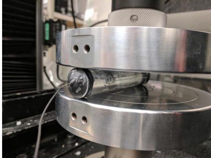
Figure 1-30: An epoxy roller with an integrated compressed FBG on the testing machine [142].
