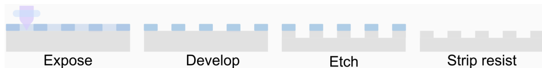
FIGURE 2.6: Spatial light modulator projects a laser light onto the wafer exposing deposited resist. The pattern is developed and etched, and the resist is stripped. In this example, a positive photoresist is used.
