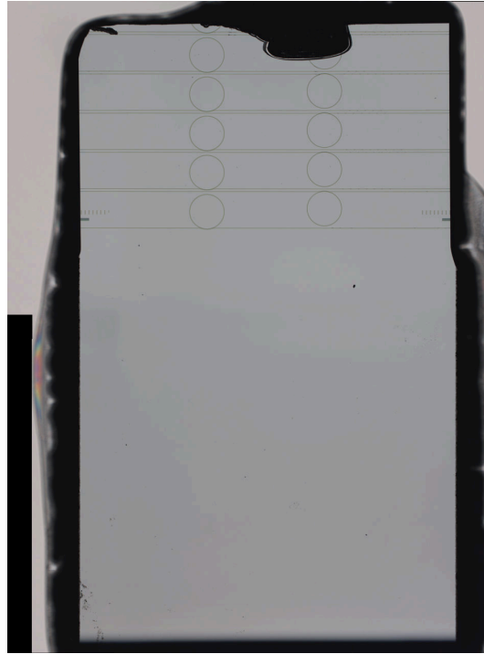
FIGURE 5.15: Microscope image of a chip with SiN waveguides spanning through the whole chip width (tapered towards the edges), enabling edge light coupling and detection.
