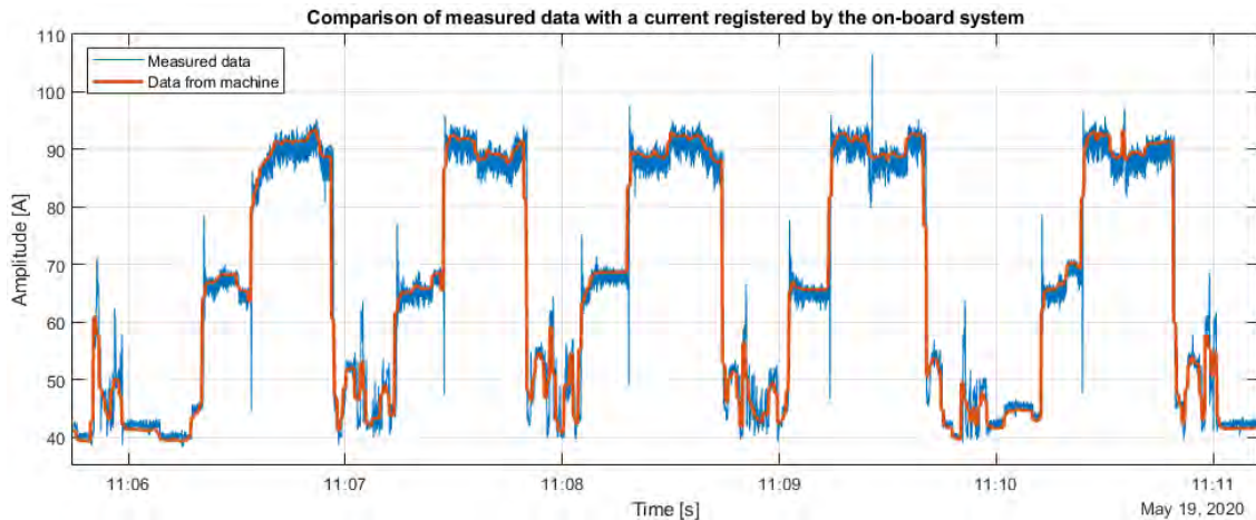
Figure 51: Electric current signal comparison with drilling rig on-board monitoring unit data [173]
