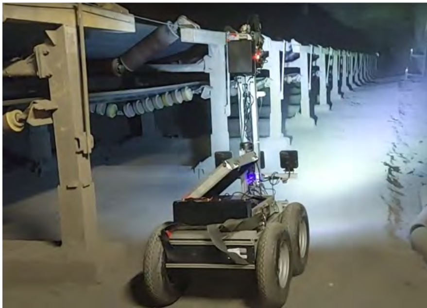
Figure 26: Robot during inspection in a mine (Source: AMICOS Project)
