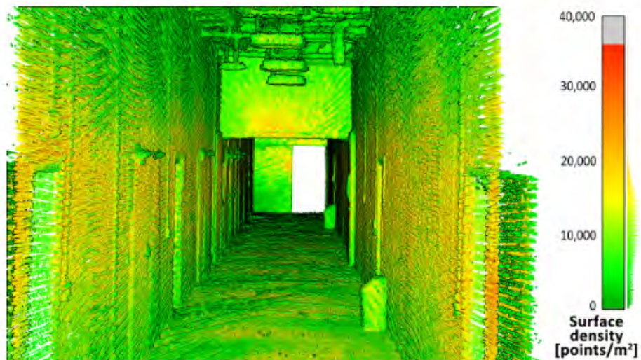
Figure 85: Point cloud density - rotating lidar [196]
