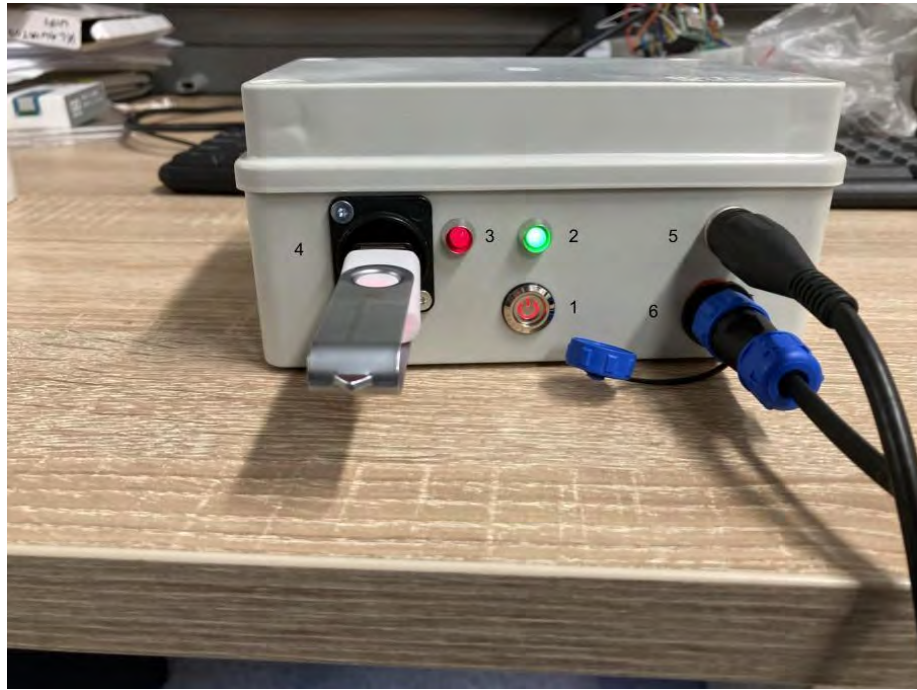
Figure 37: Current measurement device interface with a memory connected to data transfer
