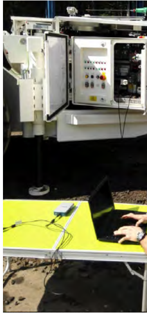
Figure 32: Standard current measurement setup during drilling rig work
