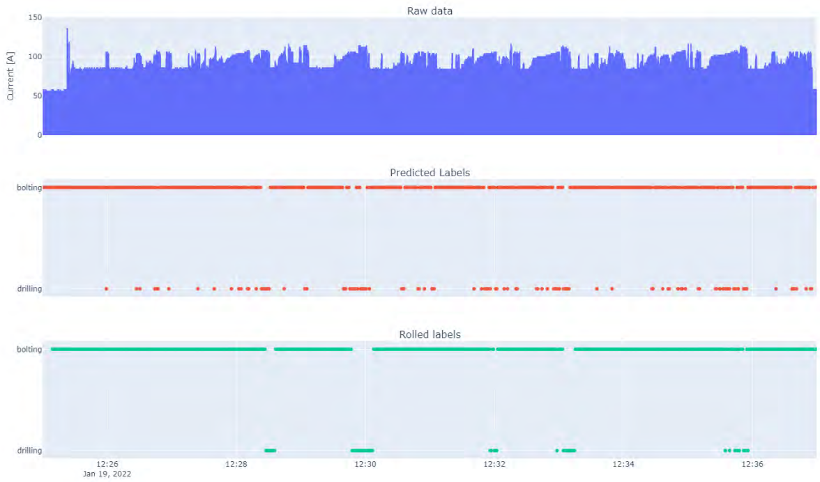
Figure 80: Predicted classess for bolting rig work phases detection using frequency bands higher than 700 Hz
