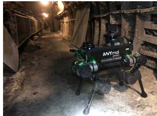
Figure 13: Legged robot for underground asset inspection [149]
