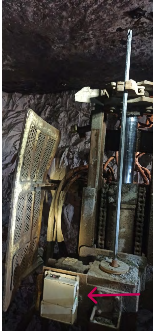
Figure 19: Laser rangefinder mounted on mining bolter boom [174]
