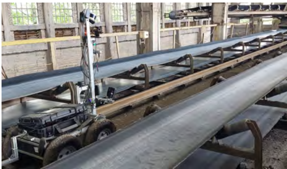
Figure 12: Wheeled robot for belt conveyor inspection [52]
