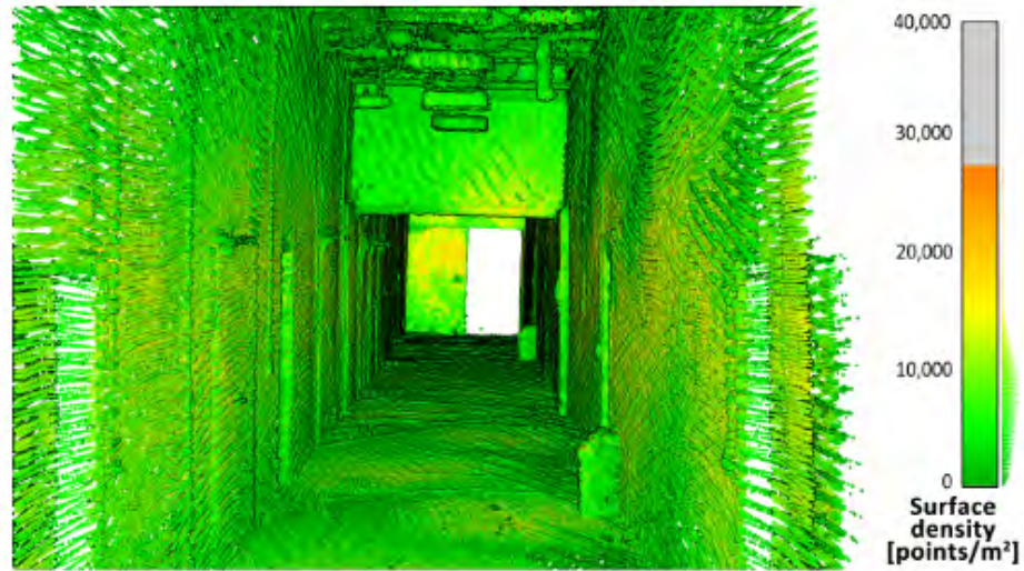
Figure 84: Point cloud density - tilting lidar [196]
