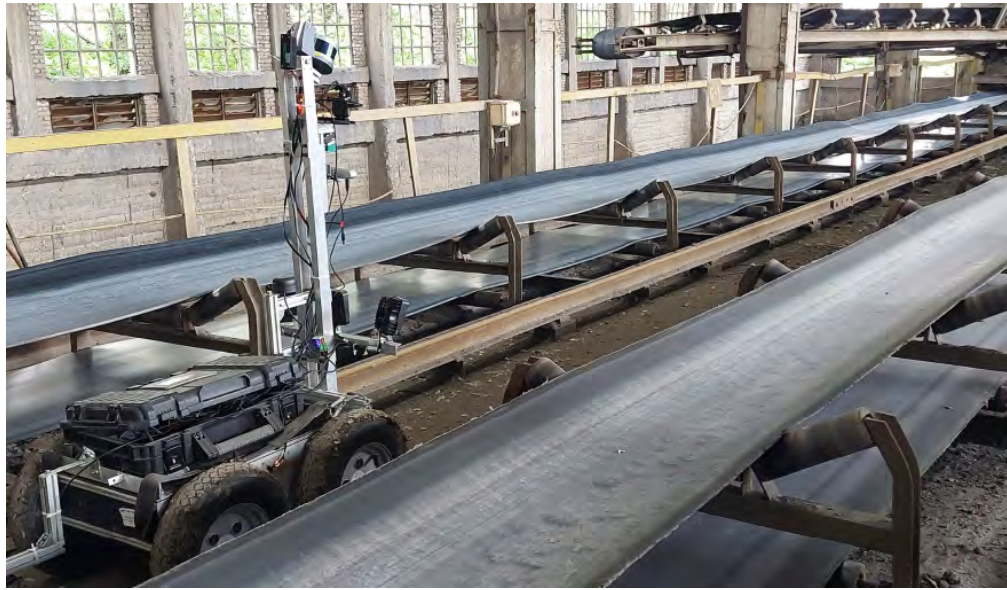
Figure 25: An automated idlers acoustic inspection with robot (Source: AMICOS project)
