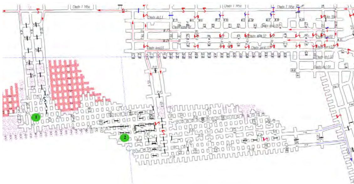
Figure 24: The map of the measurement experiment in an underground mine with sensors location and fresh and used air stream flow [175]
