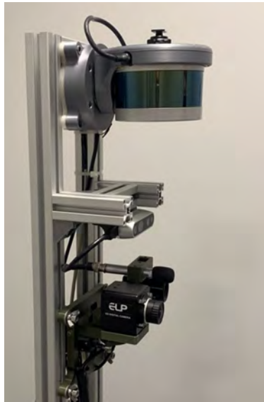
Figure 27: The view on robotic inspection sensors suite
