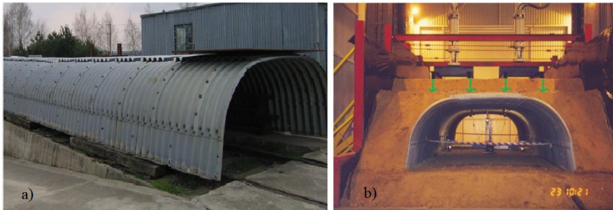
Figure 5.1: Model of the soil steel composite structure in laboratory test: a) general view of the assembled corrugated steel structure, b) after backfill model prepared for ultimate loading test [98]
