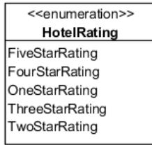
Figure 11.17 The example extracted UML Enumeration based on the selected row from Figure 11.16.
