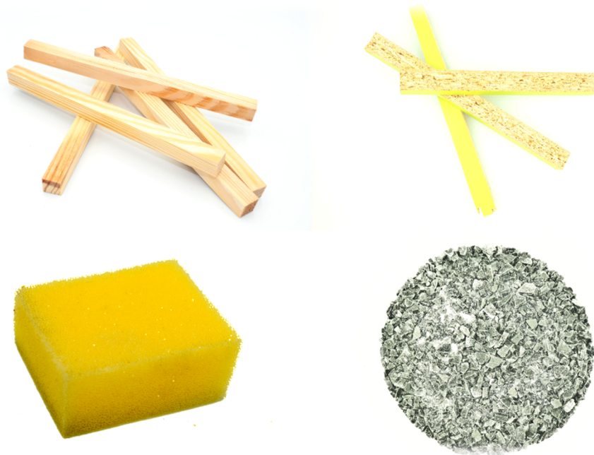
Figure 1. Four materials used in the experiment. The pinewood scantlings (PINE, upper left ), laminated particleboard (LPB, upper right ), fragment of PUR foam sheet ( lower left ), granules of PMMA ( lower right ).
