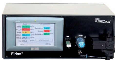
Fig. 8. An example of a Fidas200 optical aerosol spectrometer (1)
