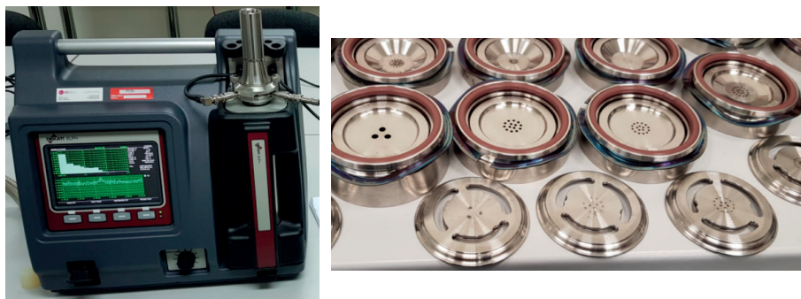
Fig. 10. Electric Low Pressure Impactor ELPI+ (3)
