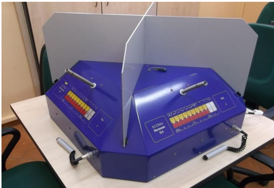
Figure 12. Dynamic olfactometer T08 by ECOMA.
