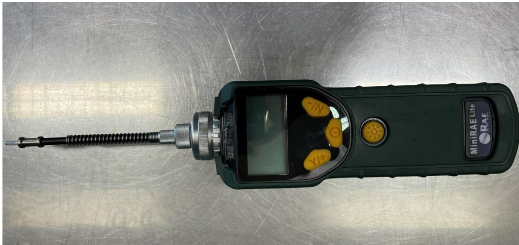
Figure 28. MiniRae Lite (PGM-7300 model) by RAE Systems.
