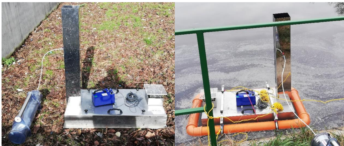
Figure 29. Sampling kit used for samples collection from area sources: biofilter on the left, landfill leachate tank on the right.
