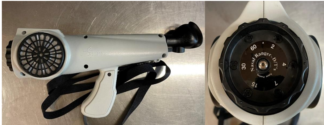
Figure 26. The used field olfactometer Nasal Ranger (on the left) manufactured by St. Croix Sensory, Inc., and the D/T dial of used field olfactometer (on the right).
