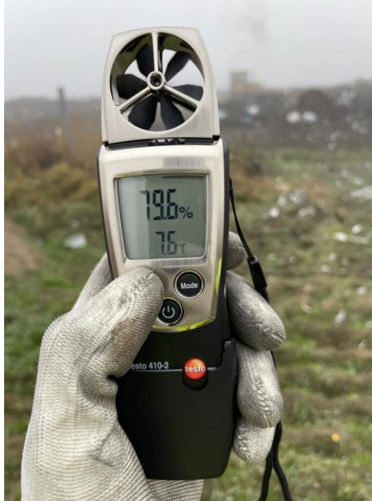
Figure 30. Testo 410-2 handheld weather station used for meteorological conditions measurements.
