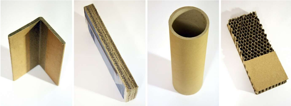
Figure 2.2. Paper-based products for architectural applications; (a) paperboard (on the example of paper L-shape); (b) corrugated cardboard panel; (c) paper tube; (d) honeycomb panel.
