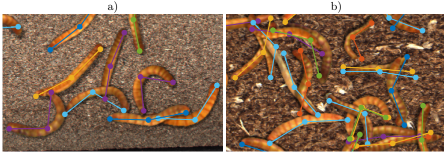
Fig. 4. Example predictions of the centerline model on images from the validation set. In low-density scenarios (a), the detector performs very well even if the instances overlap slightly. With increasing object density (b), accuracy of endpoint placement decreases, and false positive predictions (duplicates) occasionally appear.
