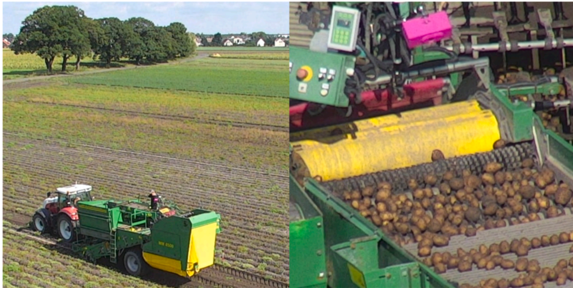
Fig. 2. Field experiment. Image acquisition system deployed during harvest (left); close-up on the system enclosed in a pink 3D-printed case (right).
