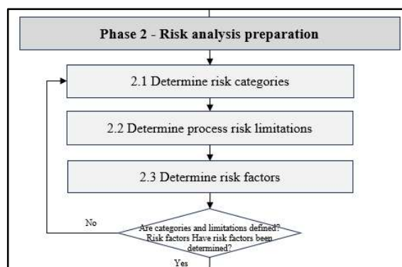
Figure 13 Phase 2 of the methodology of assessing and reducing the risk of development of tooling in automotive industry - risk analysis preparation
