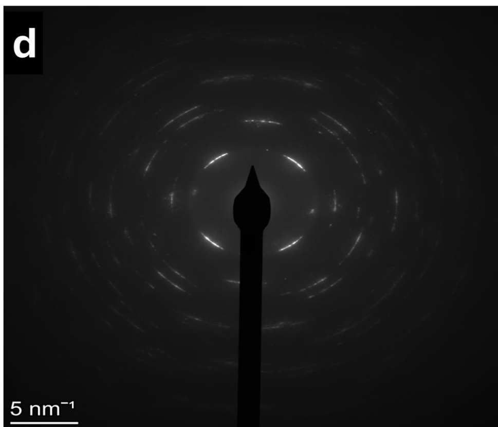
Fig. 12. Structure of the Zn-Fe-Mo alloy coating deposited from a plating bath containing (\text{NH}_4)_2\text{SO}_4 at 20 \text{ mA cm}^{-2} at 25 \text{ }^\circ\text{C} . The appearance of the lamella with marked imaging and diffraction areas (a), STEM HAADF structure (b,c) and SAED diffraction pattern (d).
