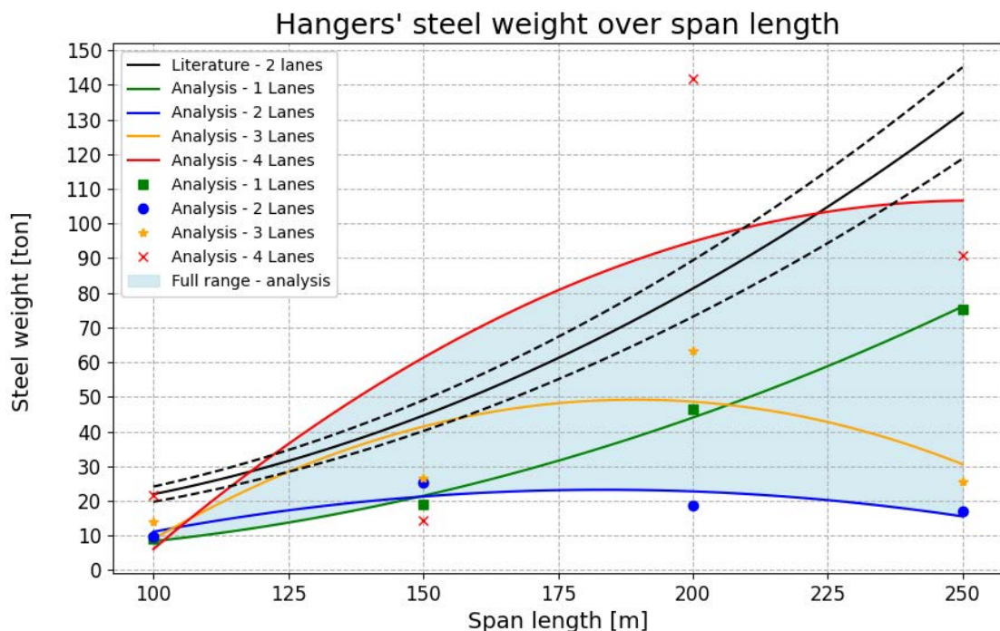
Figure 6.30 Hangers' steel weight comparison with the literature results for all the deck widths - the dashed lines represented literature weight estimation with deviation of 10%
