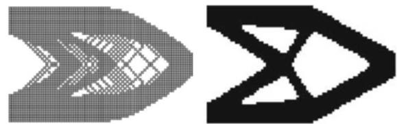
Figure A.12 Example of checkerboard pattern formation in hard-kill mechanism and fixed solution with soft-kill mechanism [121]
