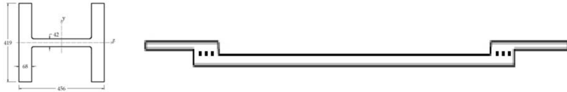
Figure 3.11 The example of proposed type of sections for the arch, UC section, and the tie, post-tensioned concrete slab [115]
