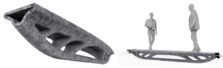
Figure A.14 Example of 3D printed post-tensioned concrete girder [118]
