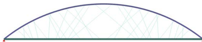
Figure D.22 The most optimized geometry for mix topology approach with prestressed steel for hangers
