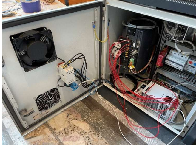
Figure 5.20. Drive system of the physical prototype of resonance punch press machine and its measurement equipment.
